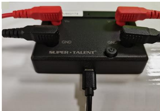
Insert Micro-B connector to Oscilloscope
